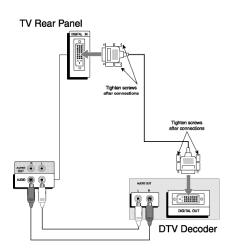
By inputting a High-bandwidth Digital Content Protection high-definition picture source to the Digital-In terminal of this television, high-definition pictures can be displayed on the screen in their digital form. (*This terminal is for use in the future when High-bandwidth Digital Content Protection DTV decoders, DVD players and D-VHS are put on the market.*)
